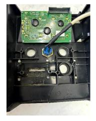
3. Place back all plastic push buttons and springs to new front panel. After fix sugar foil membrane buttons metal holder to its place.
