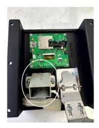
5. The new front panel is ready to place it to vending machine with 6 screws. Connect sugar buttons plugs and connect LCDs data wires to new module.
